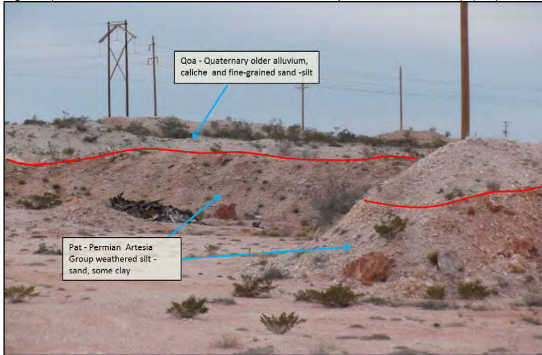
Graphic 2: Looking west at wall of caliche pit about 0.8 miles west-southwest of MWFM Pit location (see Figure 6). Three to four feet of caliche and soil exist on top of the Artesia Group (Pat).
