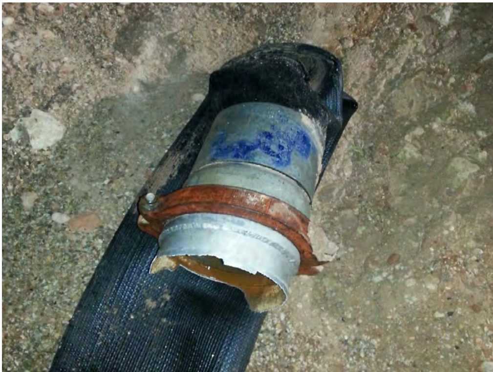
BEU-DI-9 #34H Frac Spill – Broken Flange at Point of Release
