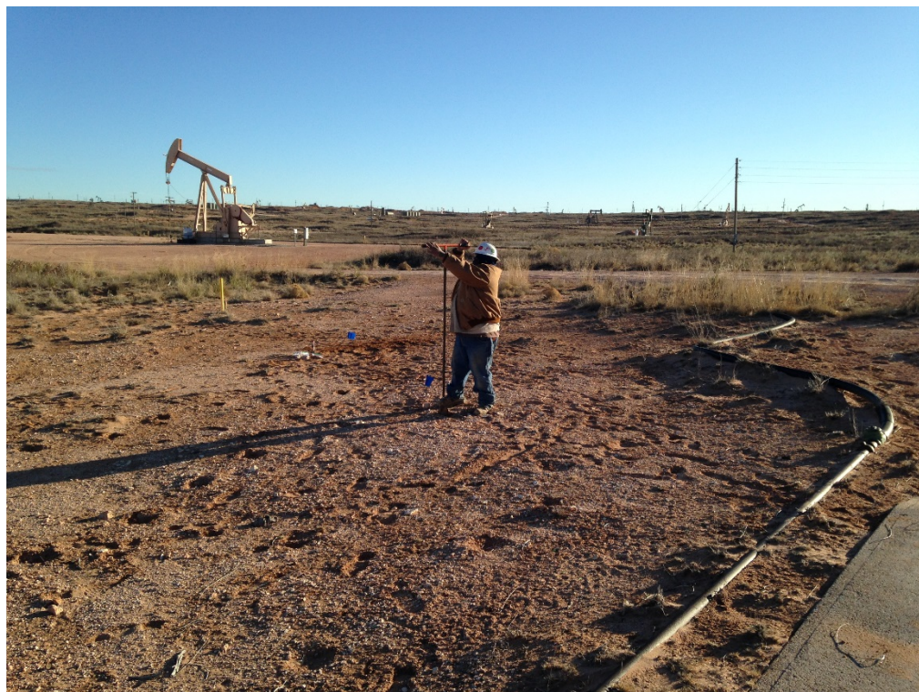
Collecting samples via auger
