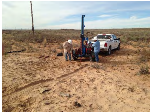
Collecting soil samples by soil bore installation, facing northwest
