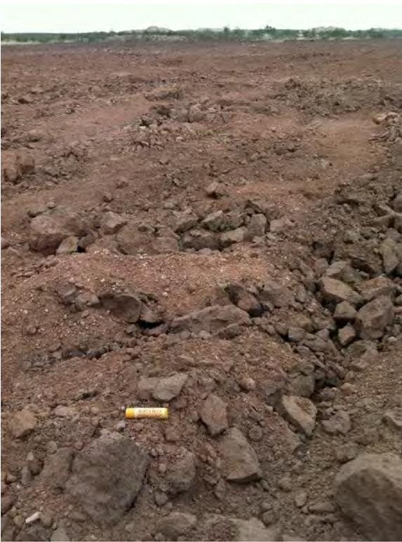
The texture of the graded surface soil within the spill footprint is a loam. Clods of dirt are clay.
