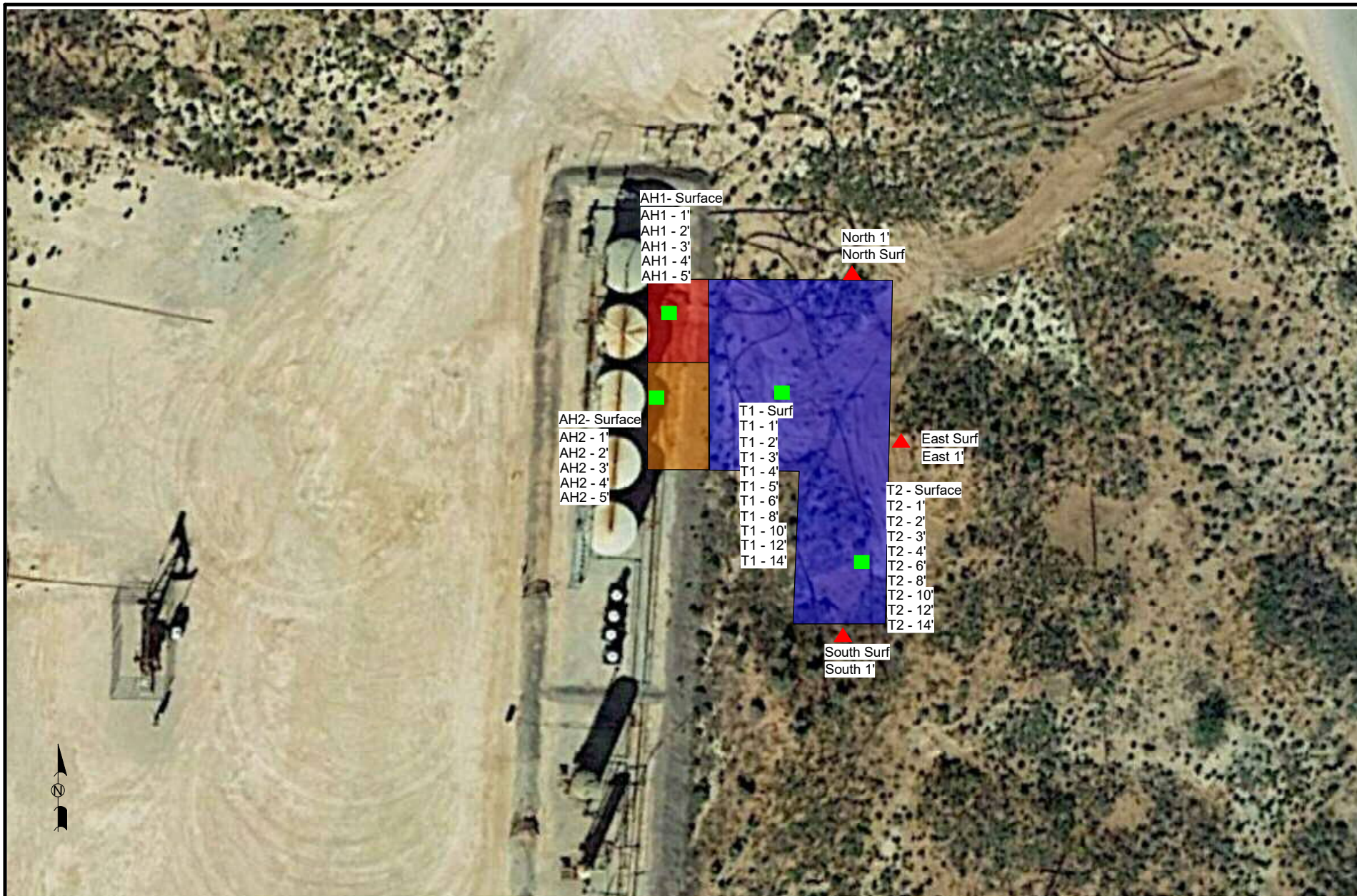
Figure 2 Site Details & Soil Sample Location Map COG Operating LLC Houma State #001 Battery Eddy County, TX
