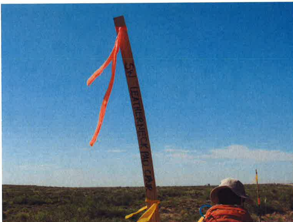
SW FRAC POND CORNER STAKE, 582397E, 3600914N
