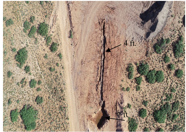
East Side Test Trench excavated to 7' bgs
