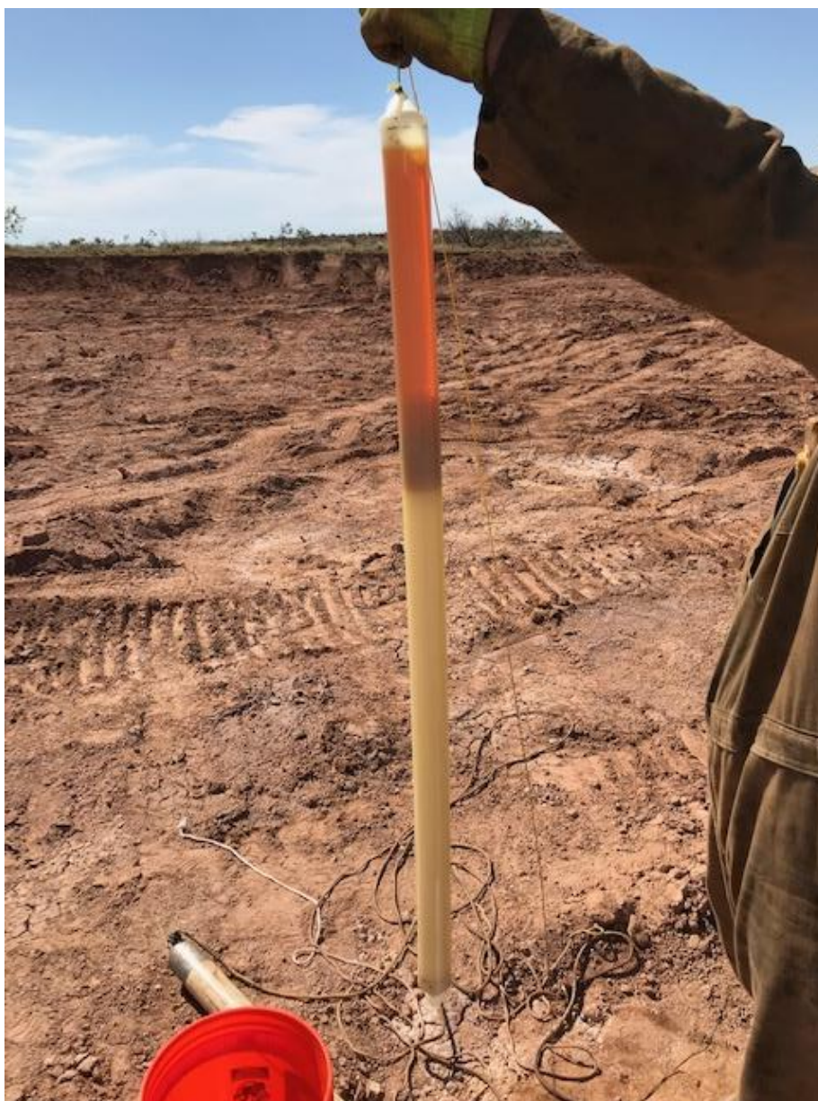
Fluid recovery in bailer from borehole BH14 (approximately 10 inches of crude oil)
