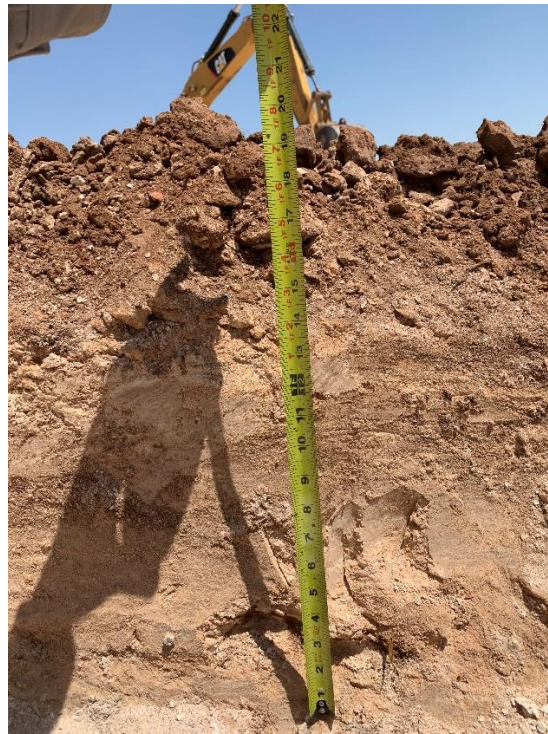
Photo 11: Area Around Electrical Pole and Burnt Surface – Test Pit showing ~20” of unconsolidated material overlying hardpan (caliche)
