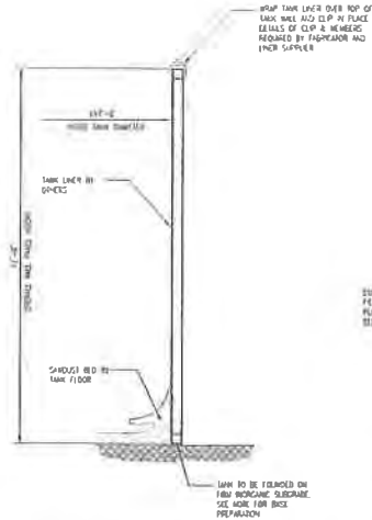
TYPICAL TANK WALL SECTION 1/2" = 1'-0"
