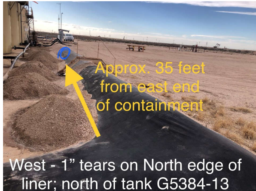
Photo 15. Location of 1-inch tears in liner on North edge of liner
