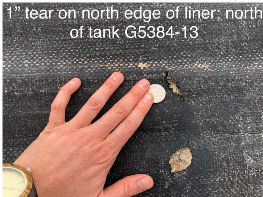
Photo 17. Size of 1-inch tears in liner on North edge of liner
