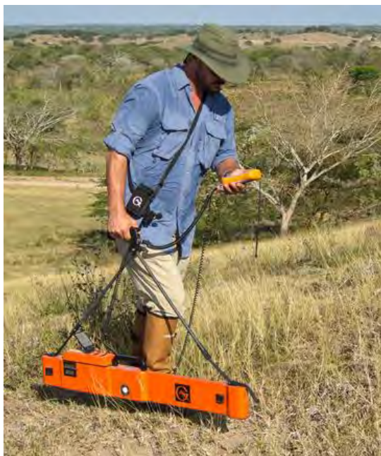
Exhibit 1: Measuring EC with the EM38 in the vertical position.
