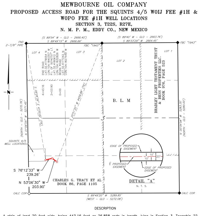
A strip of land 20 feet wide, being 443.16 feet or 26.858 rods in length, lying in Section 3, Township 22 South, Range 27 East, N. M. P. M., Eddy County, New Mexico, being 10 feet left and 10 feet right of the following described survey of a centerline across the lands of Charles G. Tracy ETAL, according to a deed filed for record in Book 86, Page 1105, of the Deed Records of Eddy County, New Mexico:
