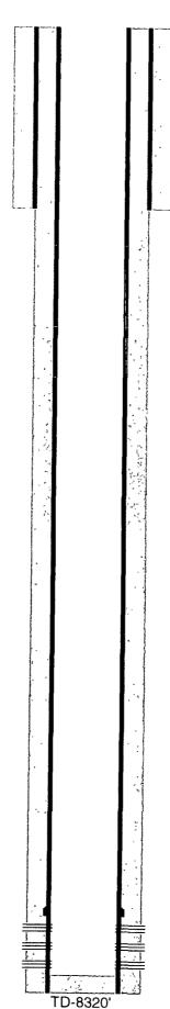
14-3/4" hole @ 1602' 9-5/8" csg @ 1602' w/ 1161sx-TOC-Surf-Circ
