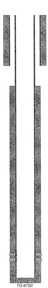
14-3/4" hole @ 1625' 9-5/8" csg @ 1625' w/ 1134sx-TOC-Surf-Circ
