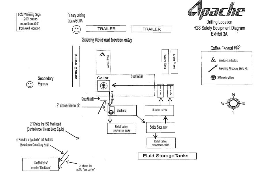
**TRAILER TRAILER** Existing Road Closed Loop Equipment Diagram Light Plant P-pe Racks Water Tank Exhibit 4 Choke Manifold — 2" choke line to pit Steel pits Shakers 2" Choke line 150' f/wellhead (Burried under Closed Loop Equip) Roll off cutting Solids Separator container on tracks 4" Panic line 150' f/wellhead (Buried under Closed Loop Equip) Roll off cutting containers on tracks Fluid StorageTanks Steel half pit
