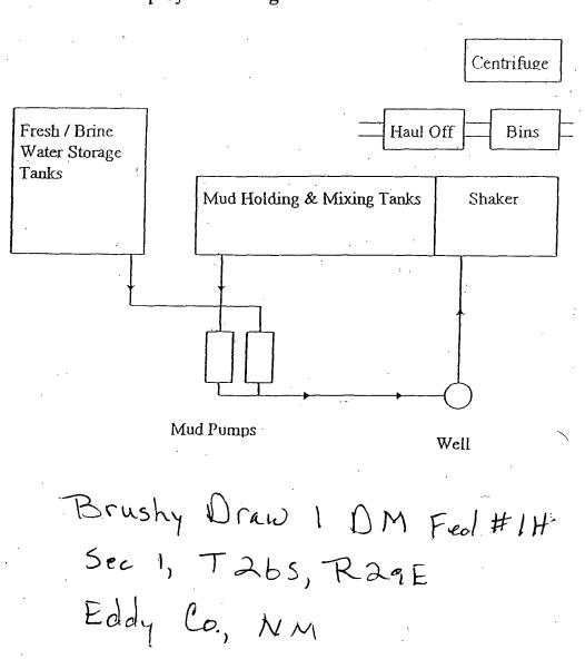
**Closed** Loop System Design & Construction
