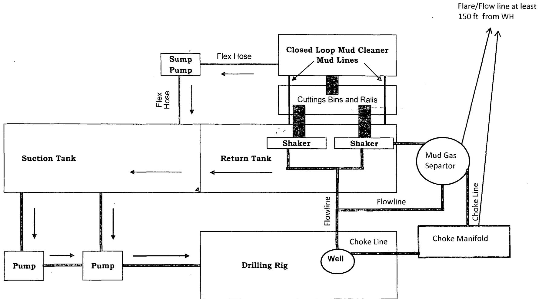
Closed Loop Pad Dimensions 385' x 300' For Pad drilling Parkway 35 Federal Com 5H and Osage 34 Federal 5H
