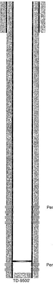
12-1/4" hole @ 1194' 9-5/8" csg @ 1194' w/ 850sx-TOC-Surf-Circ
