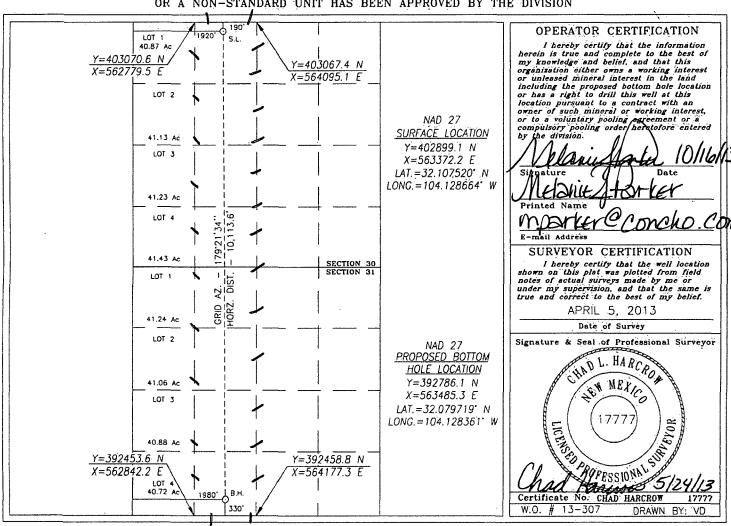
SECTION 30, TOWNSHIP 25 SOUTH, RANGE 28 EAST, N.M.P.M., EDDY COUNTY NEW MEXICO 600' **PROPOSED** MYOX 19 STATE COM #2H PAD NE COR. 170' NORTH NW COR. WELL PAD WELL PAD OFFSET 2992.4' 2997.4' 2995.4' SECTION LINE MYOX 30 STATE COM #3H 170' EAST 170' WEST OFFSET OFFSET 2993.8' 2996.1' ELEV - 2996.2'  $LAT. = 32.107520^{\circ} N$ LONG. = 104.128664° W 150' SOUTH SW COR. SE COR. OFFSET WELL PAD WELL PAD 2992.9' 2993.2' 2994.6' ALL FEATURES ARE EXISTING UNLESS OTHERWISE NOTED 600'
