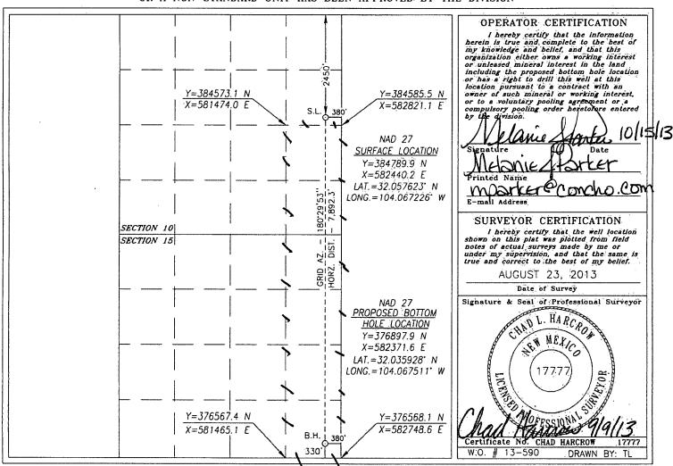
SECTION 10, TOWNSHIP 26 SOUTH, RANGE 28 EAST, N.M.P.M., EDDY COUNTY NEW MEXICO 600' 170' NORTH NW COR. NE COR. WELL PAD **OFFSET** WELL PAD 2981.2' 2983.6 2982.3' SRO STATE COM #60H 170' EAST 170' WEST OFFSET OFFSET 2981.0' 2983.3' ELEV - 2982.1 $LAT. = 32.057623^{\circ} N$ LONG. = 104.067226° W SE COR. SW COR. 170' SOUTH WELL PAD WELL PAD **OFFSET** 2980.8' 2983.1' 2981.9 ALL FEATURES ARE EXISTING UNLESS OTHERWISE NOTED 600'
