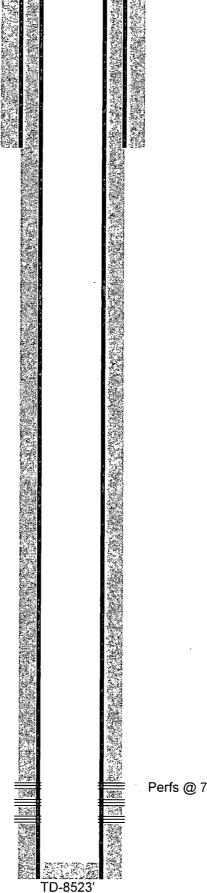
12-1/4" hole @ 1590' 9-5/8" csg @ 1590' w/ 1150sx-TOC-Surf-Circ
