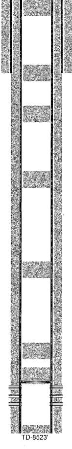
12-1/4" hole @ 1590' 9-5/8" csg @ 1590' w/ 1150sx-TOC-Surf-Circ
