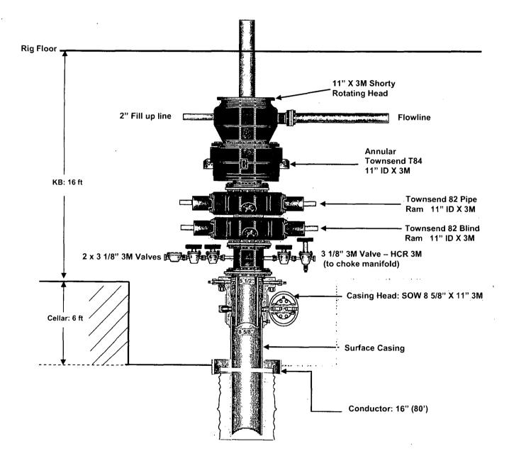
**3M CHOKE MANIFOLD CONFIGURATION**
