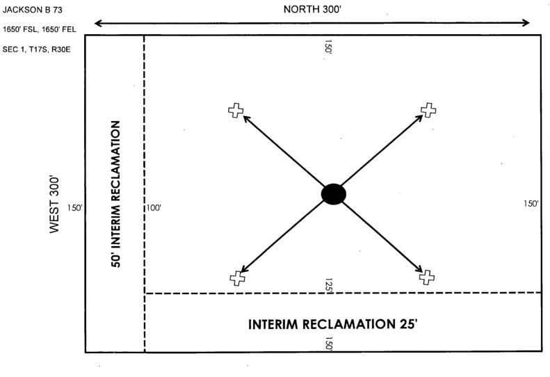
S ANCHOR 75' FROM WELLHEAD TO ANCHORS
