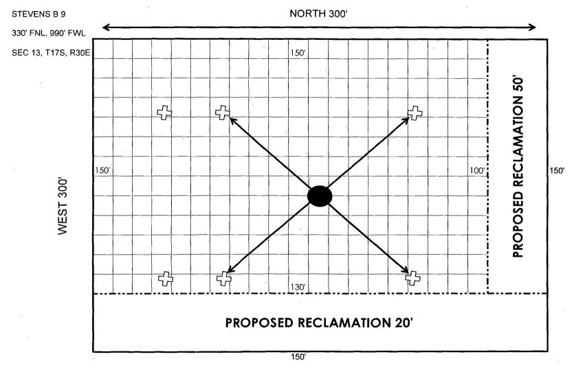
ANCHOR 75' FROM WELLHEAD TO ANCHORS
