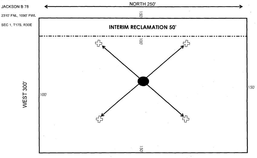
ANCHOR 75' FROM WELLHEAD TO ANCHORS
