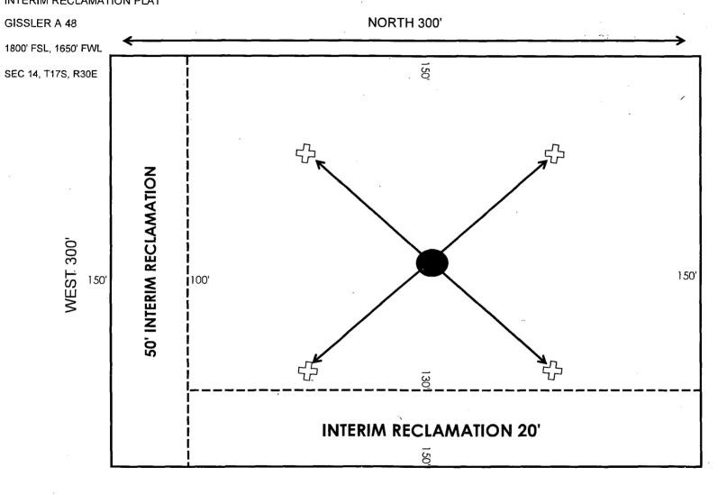
ANCHOR 75' FROM WELLHEAD TO ANCHORS
