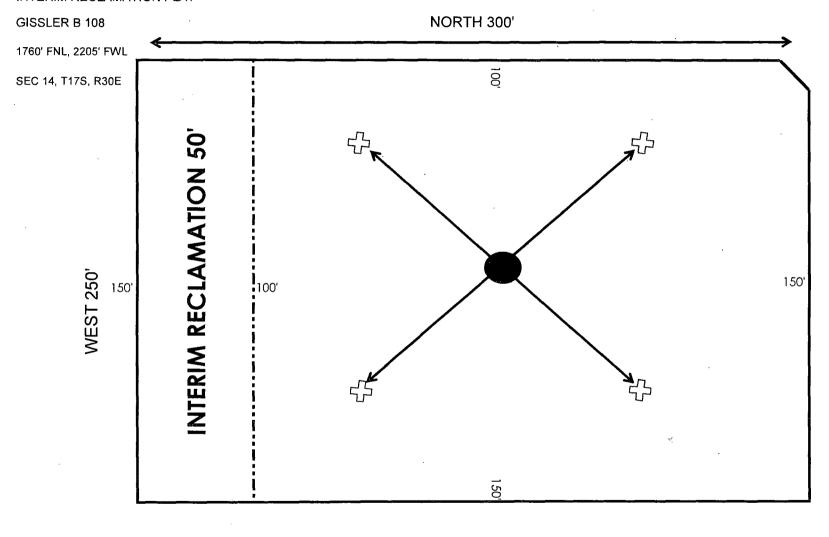
ANCHOR 75' FROM WELLHEAD TO ANCHORS
