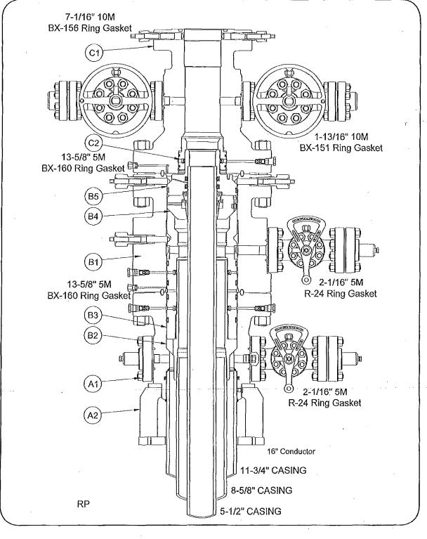
13-5/8" 5M MBS System 11-3/4" x 8-5/8" x 5-1/2" 13-5/8" 5M BOPE & Closed Loop Equipment Schematic
