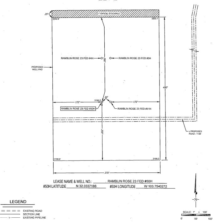
ALL BEARINGS, DISTANCES, AND COORDINATE VALUES CONTAINED HEREON ARE GRID BASED UPON THE NEW MEXICO STATE PLANE COORDINATE SYSTEM, EAST ZONE OF THE NORTH AMERICAN DATUM 1927, U.S. SÜRVEY FEET
