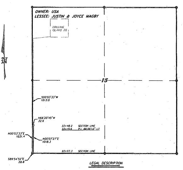
A STRIP OF LAND 30.0 FEET WIDE, LOCATED IN SECTION 15, TOWNSHIP 21 SOUTH, RANGE 29 EAST, N.M.P.M., EDDY COUNTY, NEW MEXICO AND BEING 15.0 FEET LEFT AND RIGHT OF THE ABOVE PLATTED CENTERLINE SURVEY.
