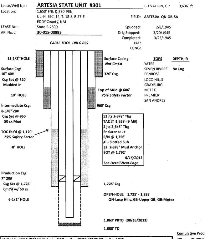
Drilled by DALE RESLER (Artesia, NM) as the JONES STATE #2 well in 1945. Re-Named the NEW MEXICO STATE "C" #3 - 10/16/68. Re-Named the ARTESIA STATE UNIT TRACT 3 #1 well - 12/01/74. Re-Named the ARTESIA STATE UNIT #301 - 06/10/2011. \* ACTUAL CUMM's 12/31/2014: 26,316 MBO, 0.244 MMCF, 43.467 MBW (NMOCD).
