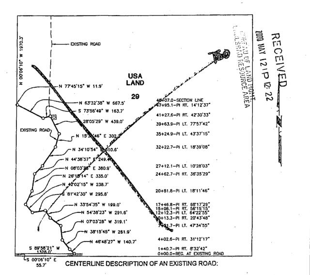
BEGINNING at a point in an existing road, from which point the southwest corner of Section 29, T-26-S, R-31-E, N.M.P.M., Eddy County, New Mexico, bears S 89° 58' 21" W, 1328.0 feet and S 00° 06' 10" E, 55.7 feet;
