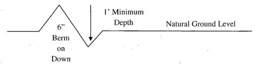
All lead-off ditches shall be graded to drain water with a 1 percent minimum to 3 percent maximum ditch slope. The spacing interval are variable for lead-off ditches and shall be determined according to the formula for spacing intervals of lead-off ditches, but may be amended depending upon existing soil types and centerline road slope (in %);
