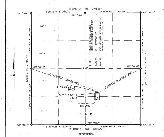
A strip of land 30 feet wide, being 162.19 feet or 9.830 rods in length lying in Section 18, Township 17 South, Range 30 East, N. M. P. M., Eddy County, New Mexico, being 15 feet left and 15 feet right of the following described survey of a centerline across B. L. M. land;
