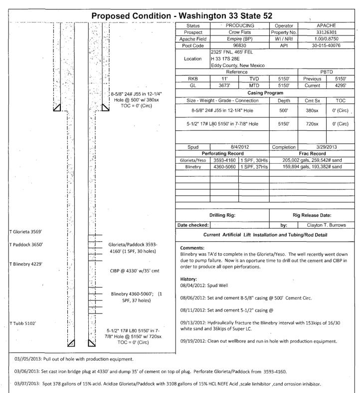
03/18/2013: Hydraulically fracture Glorietta/Paddock with 259,542 pounds of unknown sieve size sand.
