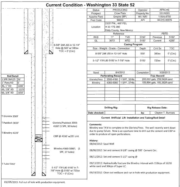
03/06/2013: Set cast iron bridge plug at 4330' and dump 35' of cement on top of plug. Perforate Glorieta/Paddock from 3593-4160.
