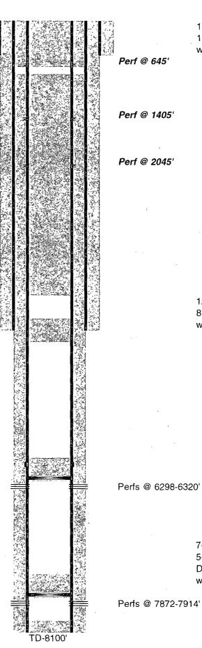
17-1/2" hole @ 595' 13-3/8" csg @ 595' w/ 795sx-TOC-Surf-Circ
