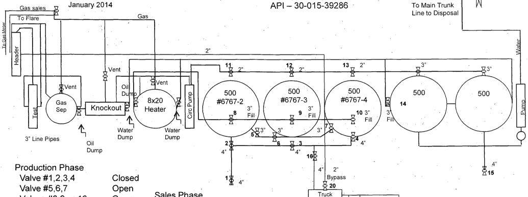
Valves #8,9 or 10 Open Valves #11.12 or 13 Open Water Line Valve #14 Open Water Truck Valve #15 Closed Valve #16 Open Valves #17,18 Closed Valve #19 Closed
