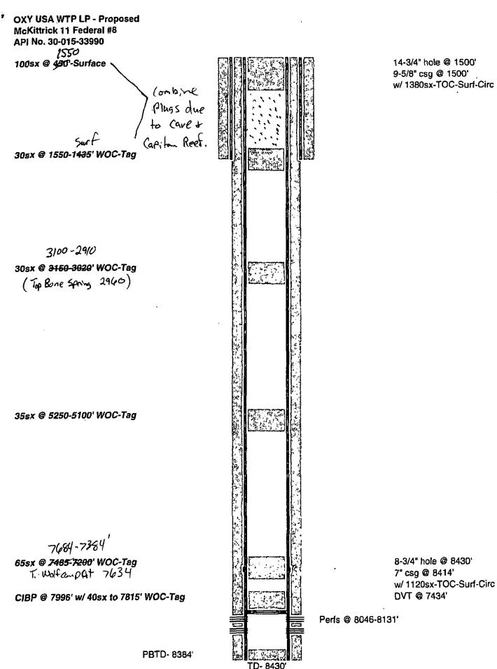
14-3/4" hole @ 1500' 9-5/8" csg @ 1500' w/ 1380sx-TOC-Surf-Circ
