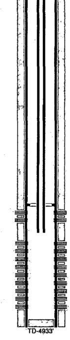
11" hole @ 409' 8-5/8" csg @ 409' w/ 360sx-TOC-Surf-Circ
