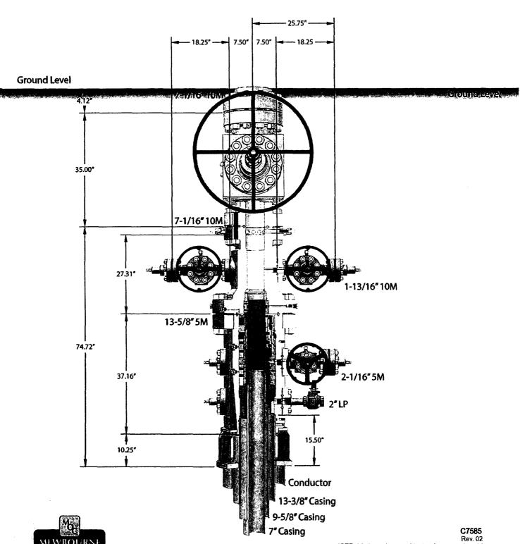
NOTE: All dimensions on this drawing are estimated measurements and should be evaluated by engineering.
