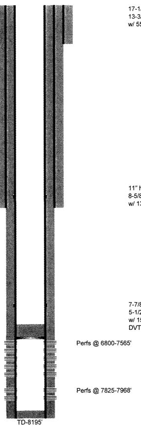
17-1/2" hole @ 812' 13-3/8" csg @ 812' w/ 550sx-TOC-Surf-Circ
