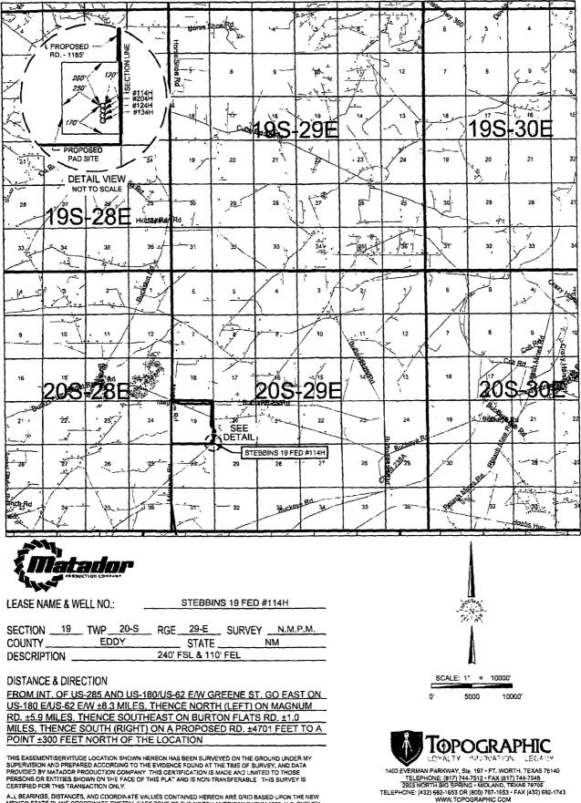
ALL BEARINGS, DISTANCES, AND COORDINATE VALUES CONTAINED HEREON ARE GRID BASED UPON THE NEW MEXICO STATE PLANE COORDINATE SYSTEM, EAST ZONE OF THE NORTH AMERICAN DATUM 1983, U.S. SURVEY FEET
