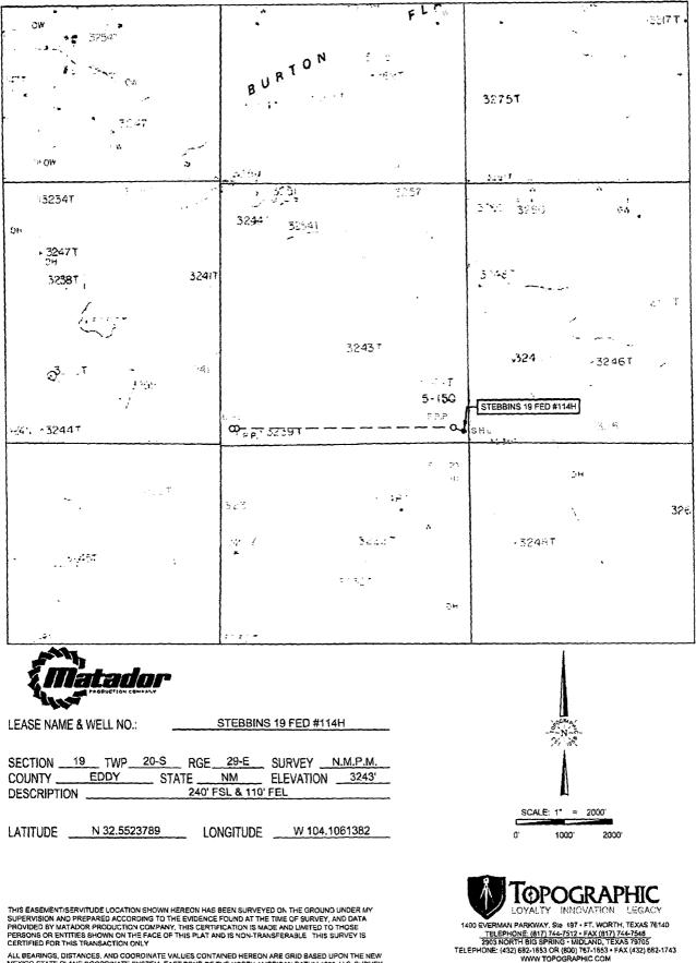
ALL BEARINGS, DISTANCES, AND COORDINATE VALUES CONTAINED HEREON ARE GRID BASED UPON THE NEW MEXICO STATE PLANE COORDINATE SYSTEM, EAST ZONE OF THE NORTH AMERICAN DATUM 1983, U.S. SJRVEY FEET
