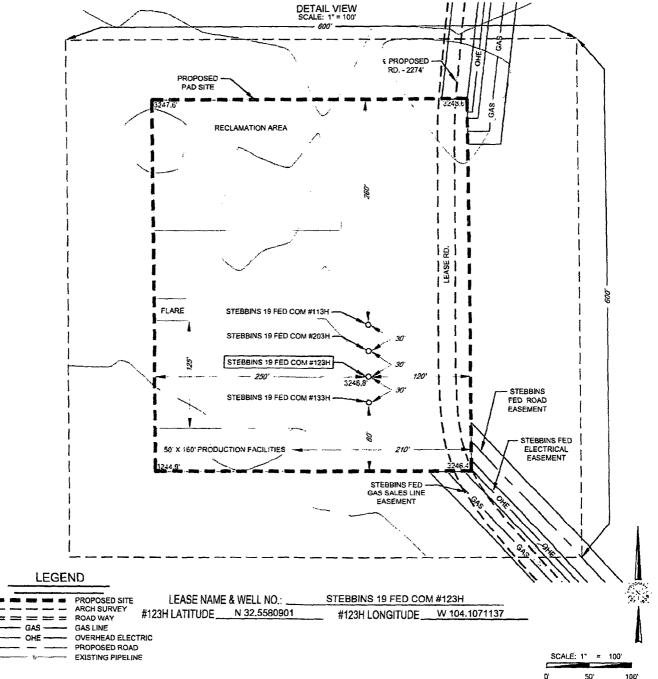
ALL BEARINGS, DISTANCES, AND COORDINATE VALUES CONTAINED HEREON ARE GRID BASEO UPON THE NEW MEXICO STATE PLANE COORDINATE SYSTEM, EAST ZONE OF THE NORTH AMERICAN DATUM 1983. U.S. SURVEY FEET
