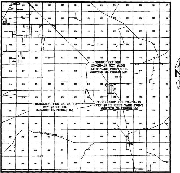
SEC. 19 TWP. 23-S RGE. 28-E SURVEY: N.M.P.M. COUNTY: EDDY DESCRIPTION: 270' FSL & 1928' FWL ELEVATION: 3084' OPERATOR: MARATHON OIL PERMIAN LLC LEASE: TREBUCHET FEE 23-28-19 U.S.G.S. TOPOGRAPHIC MAP: OTIS, N.M. SCALE: 1" = 2 MILES
