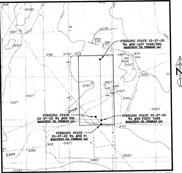
SEC. 20 TWP. 23-S RGE. 27-E SURVEY: N.M.P.M. COUNTY: EDDY DESCRIPTION: 603' FSL & 1412' FEL ELEVATION: 3181' OPERATOR: MARATHON OIL PERMIAN LLC LEASE: STERLING STATE 23-27-20 U.S.G.S. TOPOGRAPHIC MAP: OTIS, N.M. SCALE: 1" = 2000' CONTOUR INTERVAL = 5'
