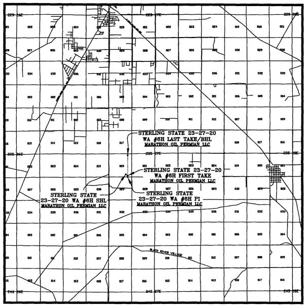
SEC. 20 TWP. 23-S RGE. 27-E SURVEY: N.M.P.M. COUNTY: EDDY DESCRIPTION: 603' FSL & 1412' FEL ELEVATION: 3181' OPERATOR: MARATHON OIL PERMIAN LLC LEASE: STERLING STATE 23-27-20 U.S.G.S. TOPOGRAPHIC MAP: OTIS, N.M. SCALE: 1" = 2 MILES
