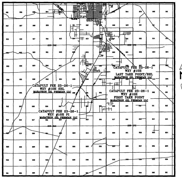
SEC. 1 TWP. 23-S RGE. 26-E SURVEY: N.M.P.M. COUNTY: EDDY DESCRIPTION: 463' FSL & 1,437' FEL ELEVATION: 3219' OPERATOR: MARATHON OIL PERMIAN LLC LEASE: CATAPULT FEE 23-26-1 U.S.G.S. TOPOGRAPHIC MAP: OTIS, N.M. SCALE: 1'' = 2 MILES
