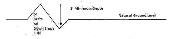
All lead-off ditches shall be graded to drain water with a 1 percent minimum to 3 percent maximum ditch slope. The spacing interval are variable for lead-off ditches and shall be determined according to the formula for spacing intervals of lead-off ditches, but may be amended depending upon existing soil types and centerline road slope (in %);
