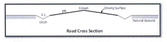
f. The access road will be constructed with a ditch on each side of the road.
