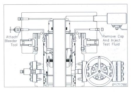
IP 0571 Page 32 Chisholm Energy 13-3/8" x 9-5/8" x 5-1/2" 5/10M MBU-3T Wellhead, With CTH-HPS-F MOD Tubing Head
