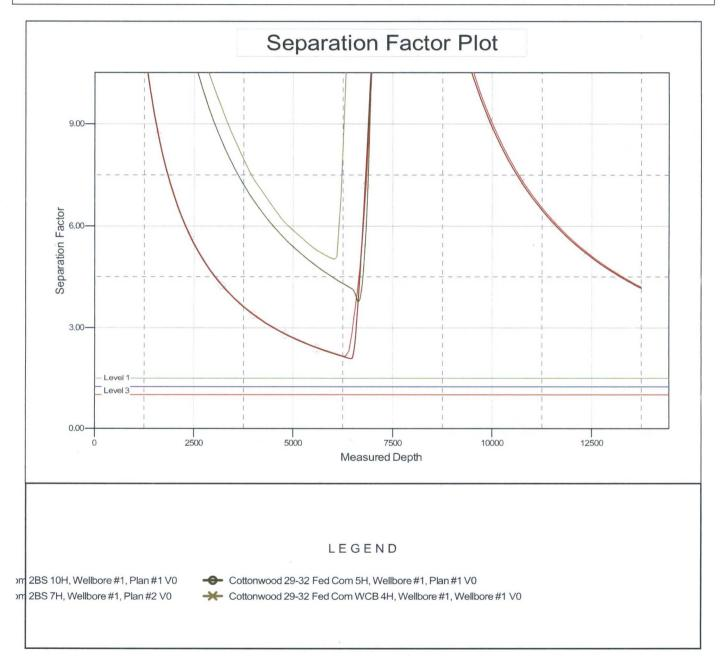
CC - Min centre to center distance or covergent point, SF - min separation factor, ES - min ellipse separation
