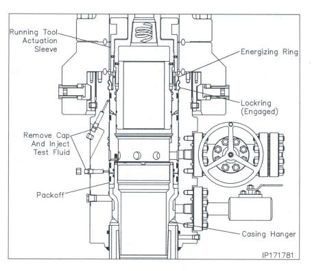
**Note:** When properly engaged the second paint mark on the landing joint will align with the rig floor. **VERIFY PAINT MARKS**.
