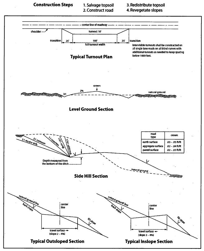
Figure 1. Cross-sections and plans for typical road sections representative of BLM resource or FS local and higher-class roads. VII. VII. DRILLING
