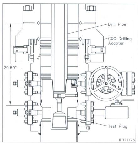
Remove as much fluid as possible from the BOP stack and the retrieve the test plug with a straight vertical lift.
