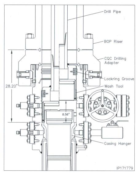
Reengage the pump and fully wash the inside of the wellhead and the entire BOP one additional cycle ensuring the stopping point is with the was tool resting on top of the hanger flutes.
