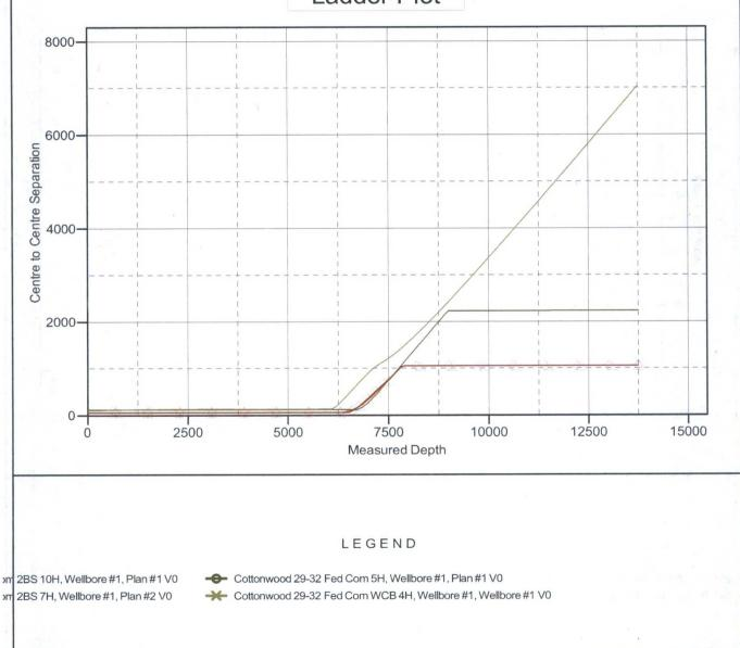
CC - Min centre to center distance or covergent point, SF - min separation factor, ES - min ellipse separation
