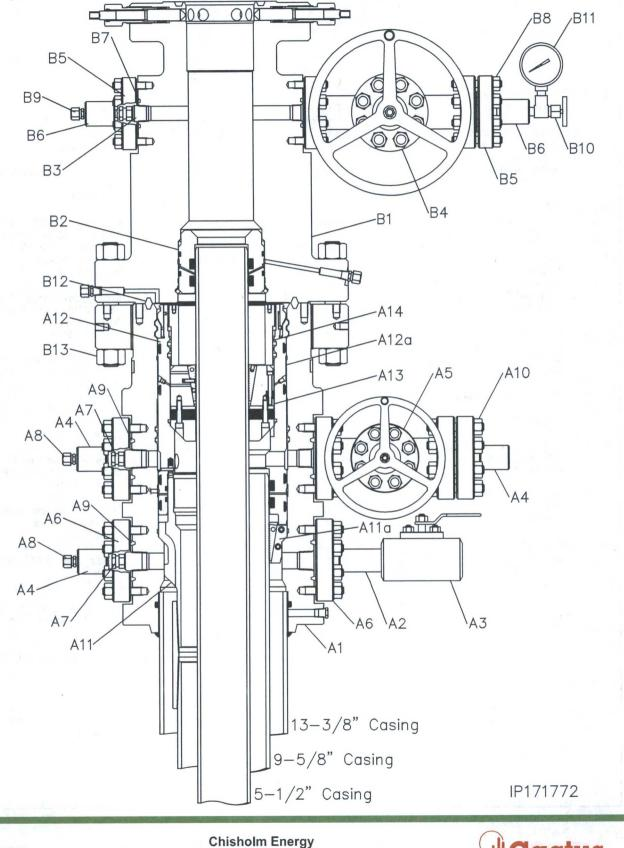
IP 0571 Page 2 13-3/8" x 9-5/8" x 5-1/2" 5/10M MBU-3T Wellhead, With CTH-HPS-F MOD Tubing Head
