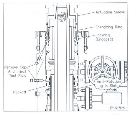
WARNING: It is imperative that the drill pipe landing joint remain concentric with the well bore when rotating to engage the lockring. This can be accomplished with the use of the air hoist.
